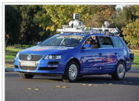
A robotic Volkswagen Passat shown at Stanford University is a driverless car
